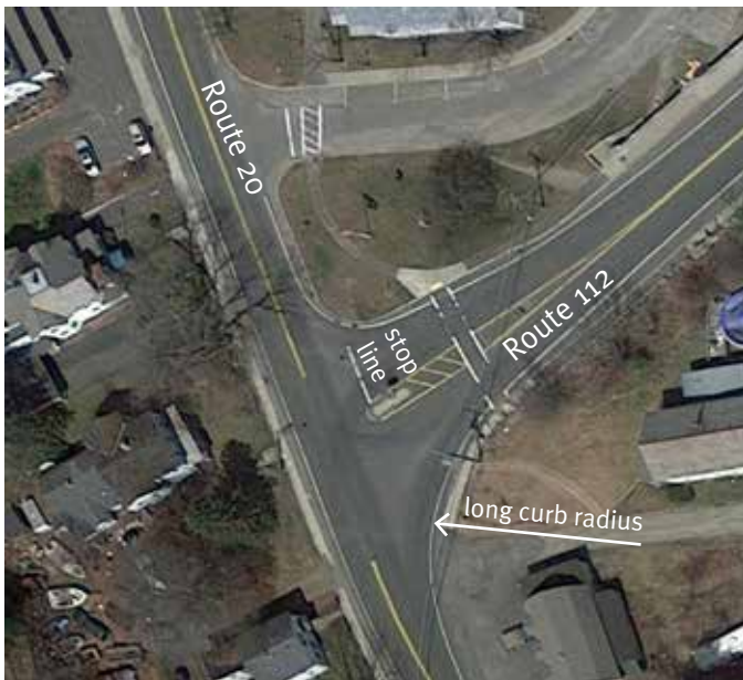
The intersection of Route 20 and 112 is precarious for pedestrians. Wide travel lanes and difficult sight lines make walkers feel vulnerable when crossing Route 112.
